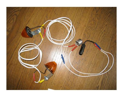
Picture 1. Shows the entire flashing light setup. TRACE THE CIRCUIT BEGINNING WITH THE POWER PLUG. RED IS "POWER".
